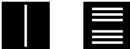
Figure 2: Two different masks needed to create MTJs.
